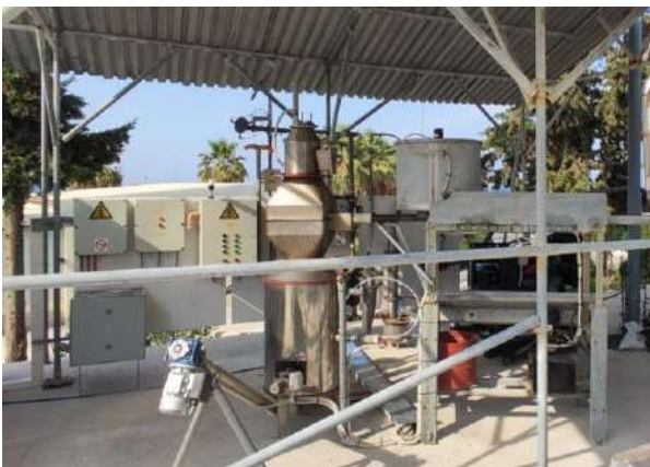
Gasification – energy production system
